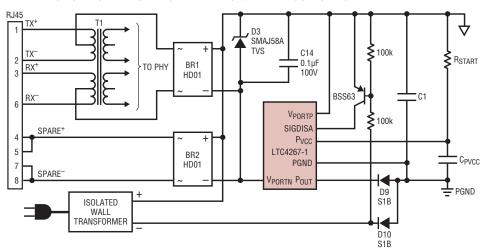
OPTION 3: AUXILIARY POWER APPLIED TO LTC4267-1 PD AND SWITCHING REGULATOR
