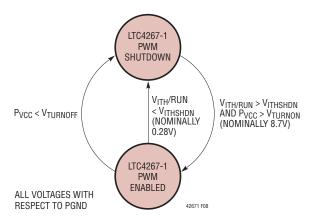
Figure 8. LTC4267-1 Switching Regulator Start-Up/Shutdown State Diagram
