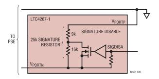
Figure 3. 25k Signature Resistor with Disable
