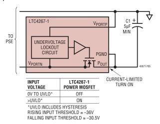
Figure 5. LTC4267-1 VPORTN Undervoltage Lockout
