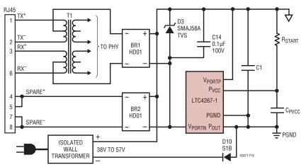
Figure 16. Auxiliary Power Source for PD
