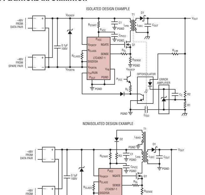
Figure 11. Typical LTC4267-1 Application Circuits
