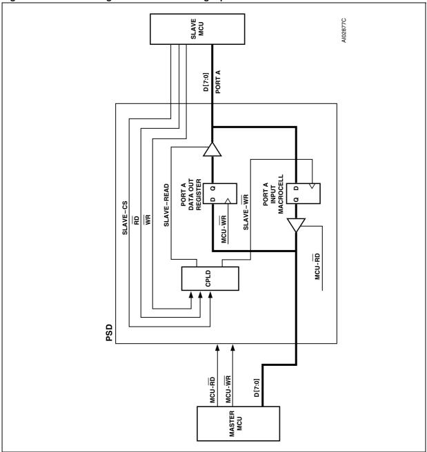
Figure 17. Handshaking communication using input macrocells
