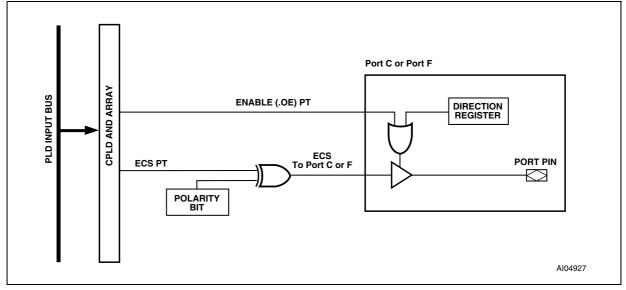
Figure 16. External Chip Select signal
