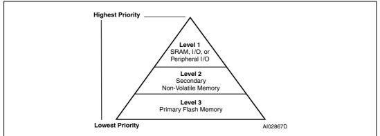
Figure 7. Priority level of memory and I/O components
