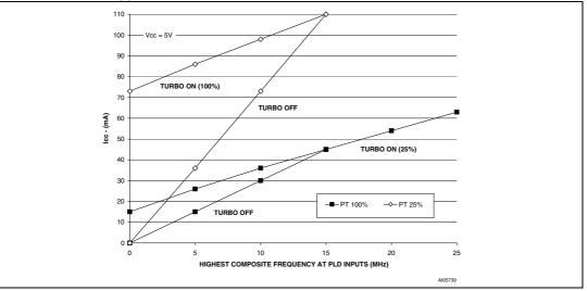
Figure 34. PLD I<sub>CC</sub> /frequency consumption
