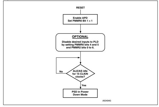
Figure 32. Enable Power-down flowchart
